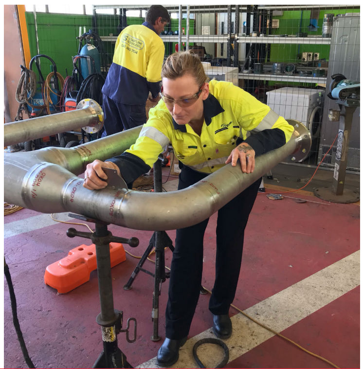
Top: Emma Claridge, Quality Assurance Advisor, UGL. Middle: Emma Claridge performs an inspection on a pipe according to ASME B31.3 Process Piping . Bottom: Emma Claridge performs an inspection on a pipe according to ASME B31.3 Process Piping .
