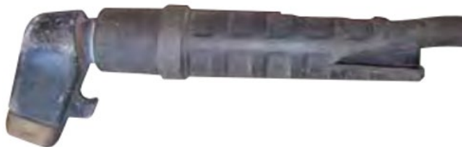
Figure 4.8 Damaged electrode holders should not be used
